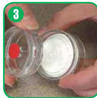
Complete cassette assembly. After sampling, remove Accu-CAP from cassette and weigh.
