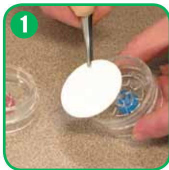
Prepare SKC 2-piece cassette with support pad.
