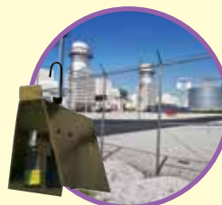
Fenceline monitoring (up to 24 hours) with UMEX 200 and shelter
