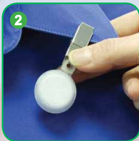
Clip in worker's breathing zone to sample.
