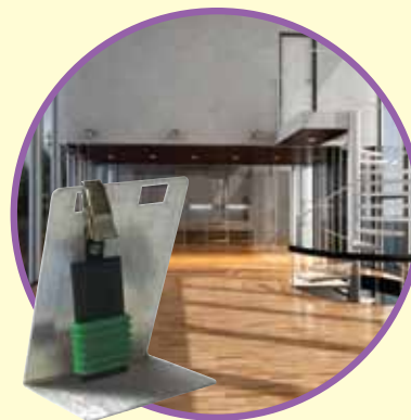
Convenient indoor air formaldehyde sampling (24 hours or 7 days) with UME x 100 and stand accessory
